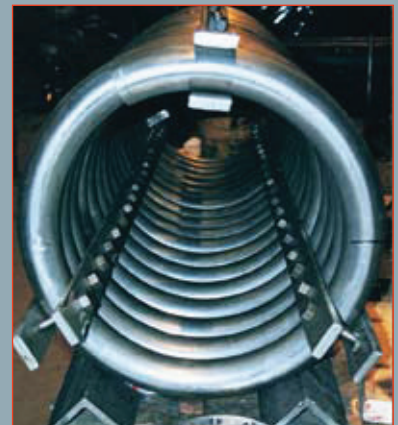
2" Sch 80 Inconel 800HT Superheater for High Pressure Air Atomizer
