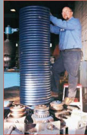
1" Sch 80 x 50 turn spiral steam coil
