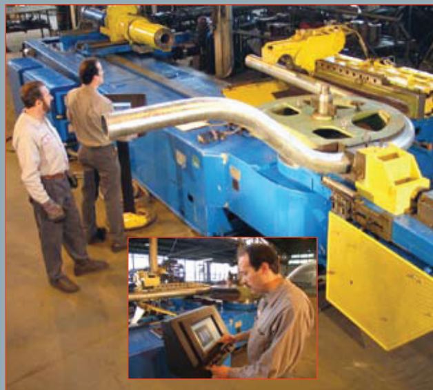
CNC Bending to 8" Schedule 80 Pipe
