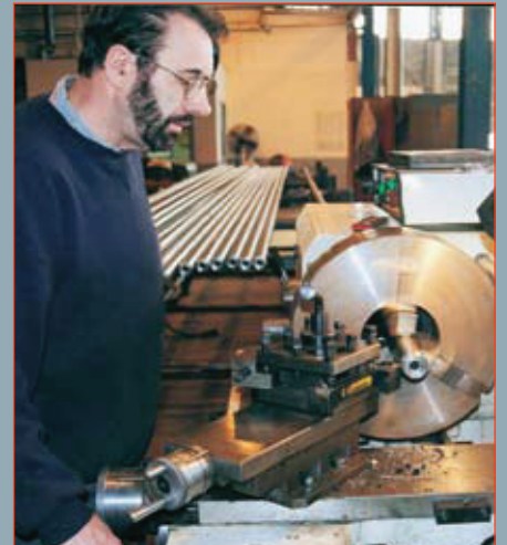
End prepping stainless tube for welding
