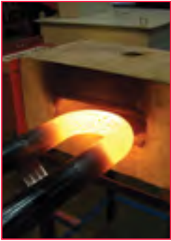
Induction Heater for Hot Bending
